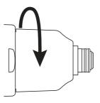
2 Turn the torque adjustment ring counterclockwise to remove
