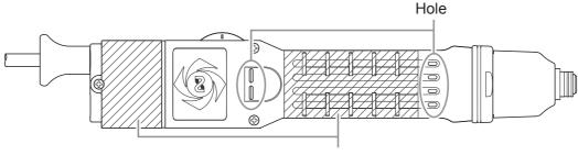
Fixing position of fixing jig
