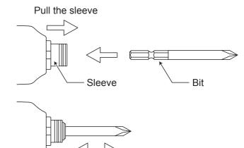
2 Release the sleeve and make sure the bit does not come off
